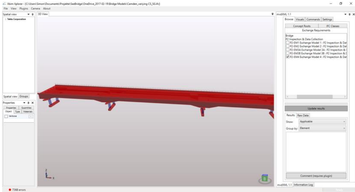
Figure 6. Checking an IFC bridge model for compliance with the defined MVD using XBIM Explorer
